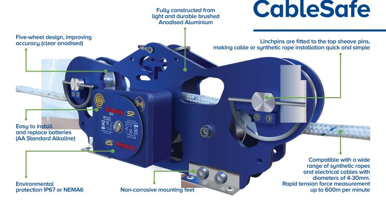
In addition to the TIMH range, the CableSafe is the continued evolution of Straightpoint's running line tensiometers. When used in the field, it will allow the user to monitor tension with exceedingly high levels of accuracy, which ensures rope/cables do not become overstretched or break.
