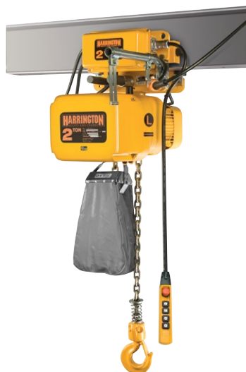
NERM/ERM020L-L/S (Shown with optional canvas chain container)
