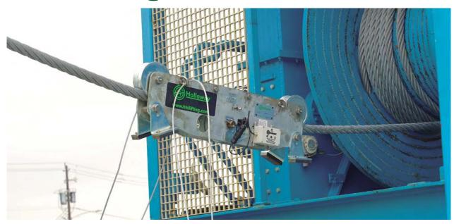
Holloway offers a diverse selection of running line tensioners, both for rent and purchase, designed for precise load monitoring in demanding marine and offshore environments. Engineered by industry experts, these tensioners deliver exceptional accuracy and corrosion resistance.
