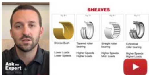
Ep. 27 Sheaves: bronze bushing vs roller bushing
